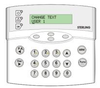
Use the scroll keys to display the change text options. You can change the following When the required user is displayed the text can be changed by using the number keys 1 to 9:
